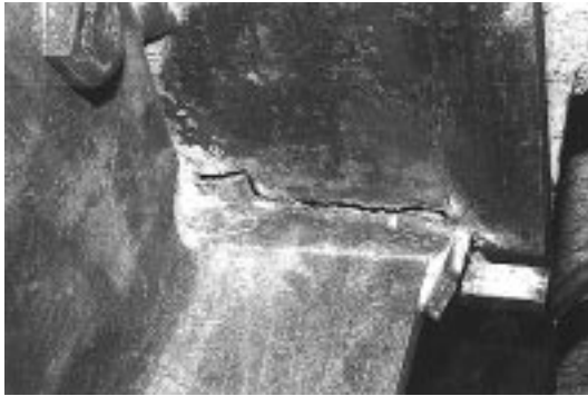
a. Fracture at Fused Zone
