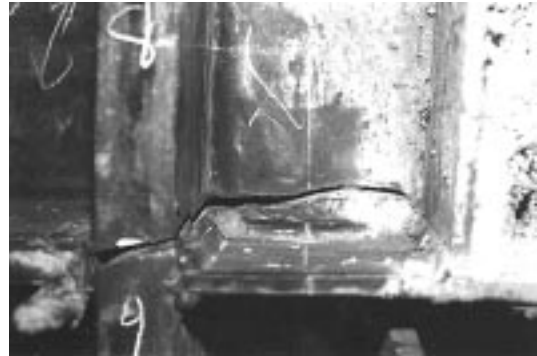
b. Fracture Progresses into Column Web
